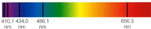
c This spectrum shows absorption lines produced by upward transitions between level 2 and higher levels in hydrogen.
