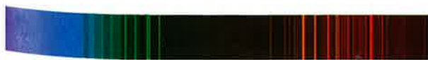
b This spectrum of molecular hydrogen ( H_2 ) consists of lines bunched into broad molecular bands.
