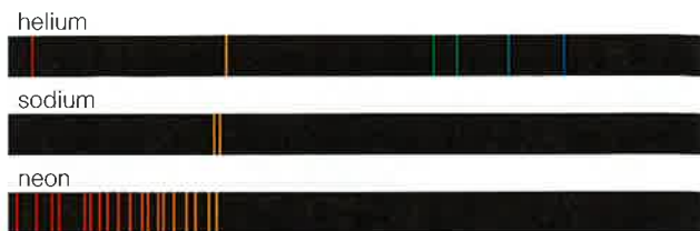
FIGURE 5.16 Visible-light emission line spectra for helium, sodium, and neon. The patterns and wavelengths of lines are different for each element, giving each a unique spectral fingerprint.
